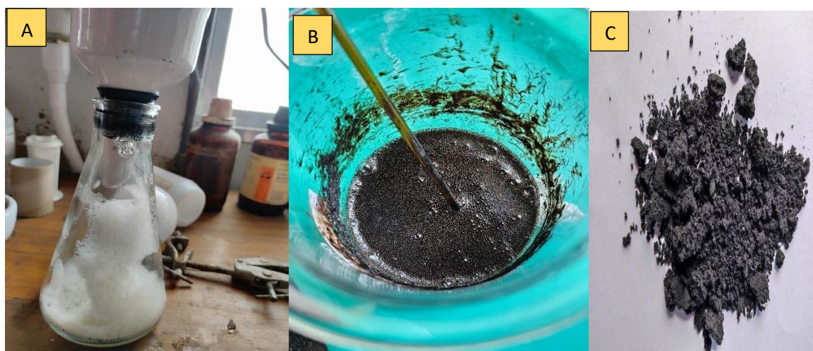
Fig 2: A: Filtration apparatus, B: Hair in KOH Solution, C: Polymerized Product
