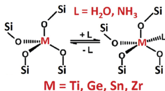
Scheme 2 Local environments of T^{4+} heteroatoms (M) incorporated into zeolitic frameworks. Vacuum-activated materials experience a Td-like environment with four equivalent M–O distances. Upon interaction with ligands ( L = H_2O or NH_3 ), the T^{4+} -atom modifies its local environment coordinating one ligand molecule in its first coordination sphere. Reprinted from ref. 8, Copyright (2014), with permission from Elsevier.
